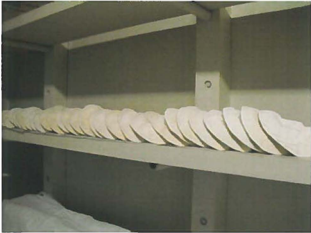
Figure 24. Annaliesa Connor-Meissner. Manner in which faces were arranged in kiln for bisque firing.
