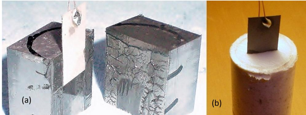
*Figure 8.* - Two methods to form the anchoring medium, casting blocks (a) and lard surface (b). Epoxy is poured into a housing that rests upon either of these horizontal surfaces. Care is taken to ensure a level casting surface that resists bonding with the anchoring medium. Any type of housing may be used in conjunction with the casting surface. Consistency in housing dimensions is recommended.
