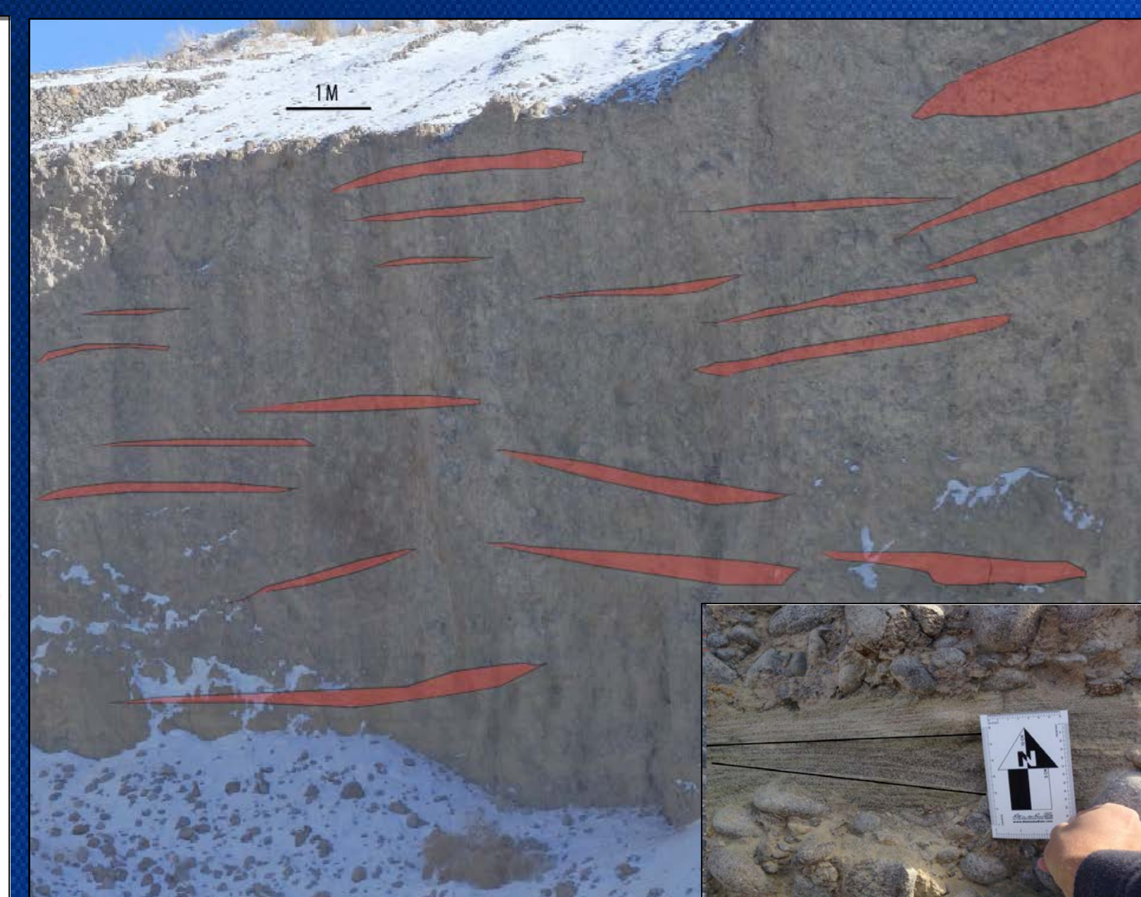
Figure 3. Map of pit wall highlighting lenses of fine grain material. Inset picture showing sedimentary structures.
