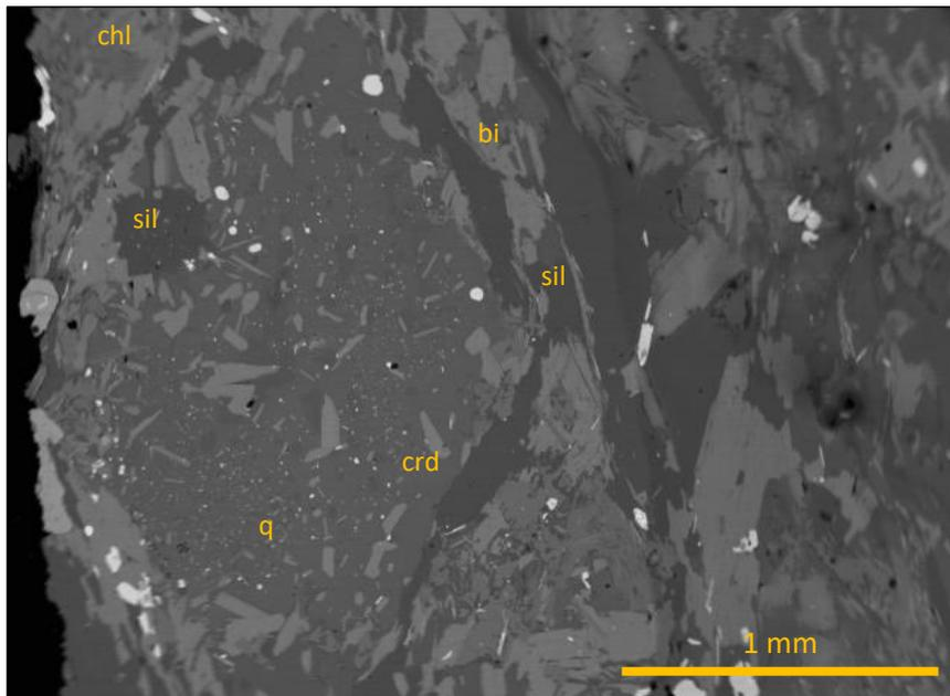
SITE 5. (Top) photomicrograph with polarized light. (Bottom) BSE – Image. 1 mm scale bar.
