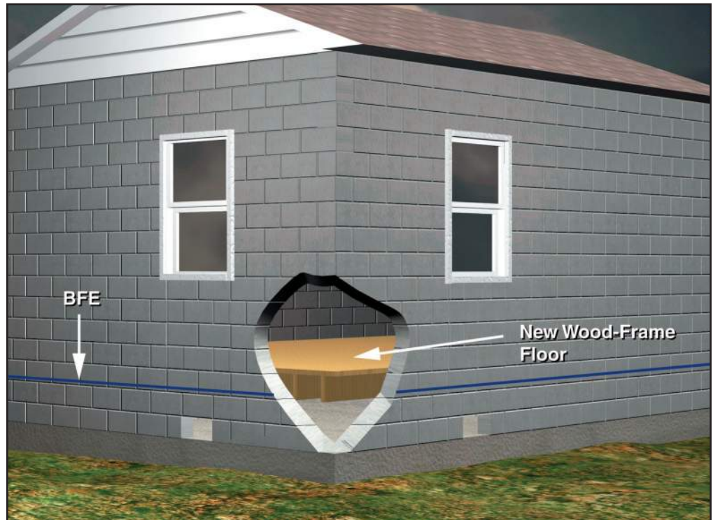
Figure 13 A new wood-frame lowest floor is constructed above the flood level, and the roof, windows, and doors are reinstalled.
