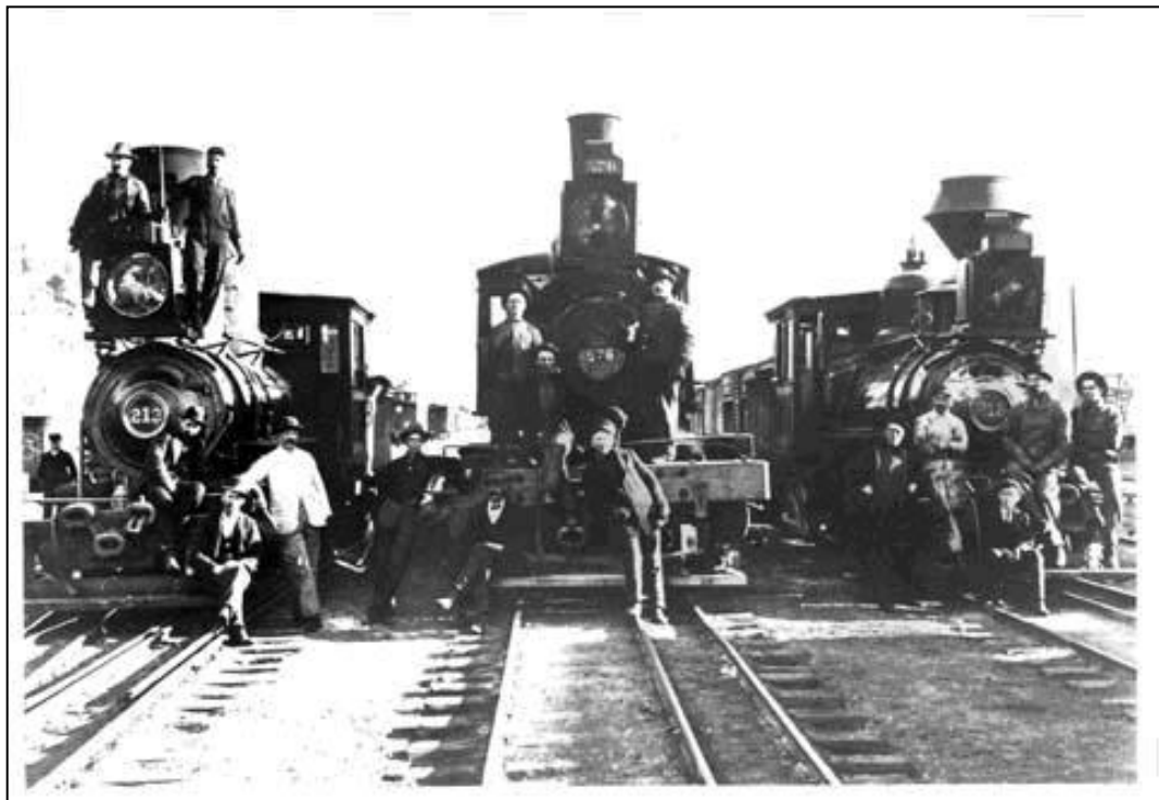
Line-up of three switch engines in Salida in 1890: no. 213 (on the left) was a narrow-gauge, no. 576 (in the center) was a standard-gauge and no. 218 (on the right) was another narrow-gauge. The D & RG seldom purchased new switch engines and used old, small, or surplus road locomotives that were converted for switching duty by adding front and rear footboards, as well as rear headlights, as these three locomotives show.
